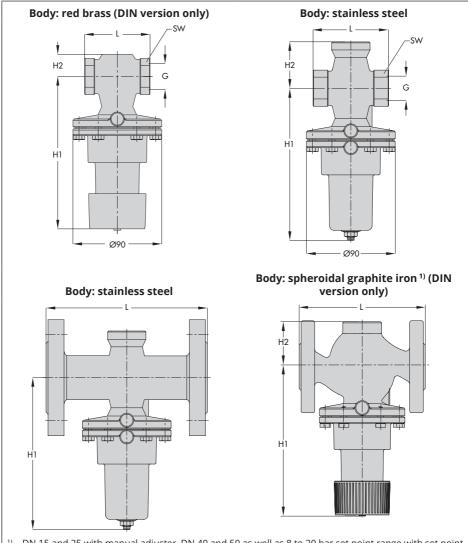
$^{1)}$  DN 15 and 25 with manual adjuster, DN 40 and 50 as well as 8 to 20 bar set point range with set point screw.
