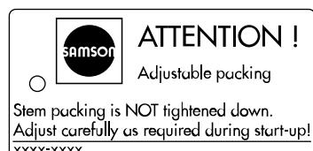
Fig. 3: Label when an adjustable packing is installed
