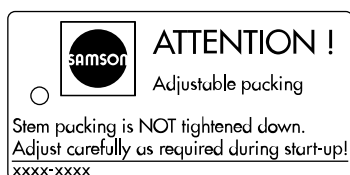
Fig. 3: Label when an adjustable packing is installed
