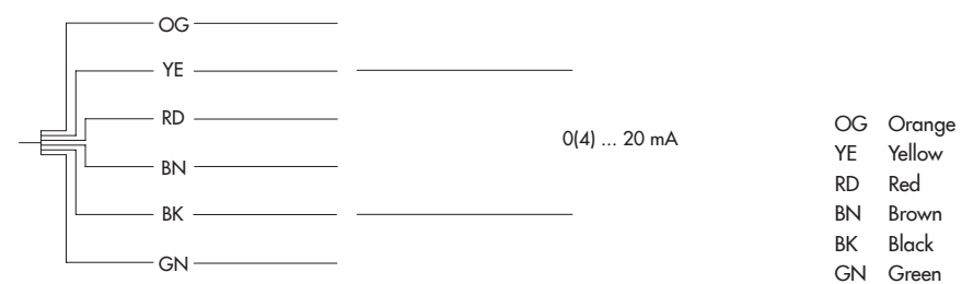
Fig. 8: Electrical connection of TROVIS 5757-3 · Control line
