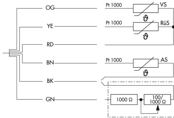
Application with flow sensor (VS), outdoor sensor (AS), binary input to switch between operating mode and potentiometer for adjusting the set point
