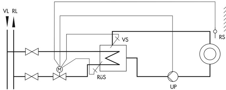
Fixed set point control with room sensor with return flow temperature limitation;
