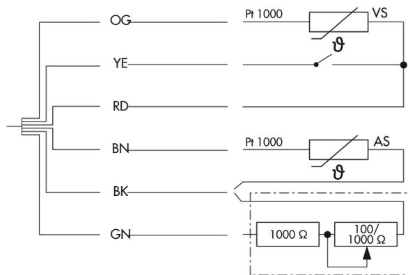
Application with flow sensor (VS), return flow sensor (RüS) and outdoor sensor (AS) and binary input to switch between operating modes
