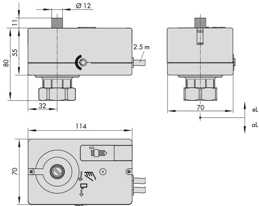
**Fig. 8:** Dimensions in mm · TROVIS 5757-7 Electric Actuator with Process Controller
