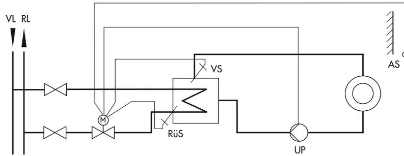
Outdoor-temperature-compensated flow temperature control with return flow temperature limitation;
