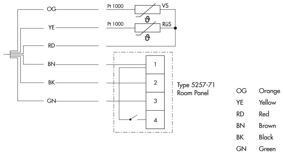
Fig. 7: Electrical connection of TROVIS 5757-7 · Control line (part 2)
