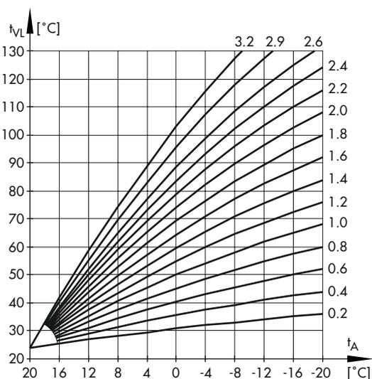
**Fig. 3:** Heating characteristics · Correlation between outdoor temperature ( $t_A$ ) and flow temperature ( $t_{VL}$ ) in the outdoor-temperature-compensated control
